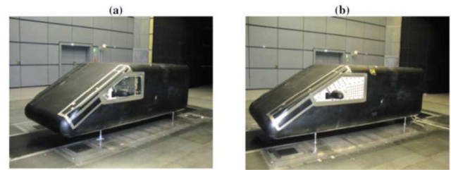
Figure 3. Wind-tunnel test: (a) glass module, (b) sensor module
